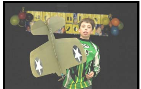
Chris Hass – Z planes P-40 A single servo powers both the left aileron and elevator. Same on the right side. Himax 4200 with a 6.6:1 gear.
