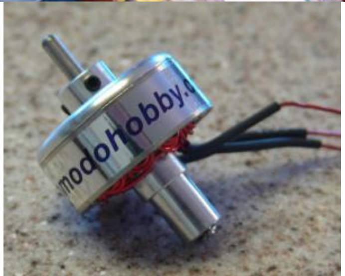
Less than three hours of work later, a 6 turn 400+ watt speed wind motor for less than $25.
