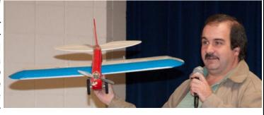
1913 Curtis Flying F Boat – John Hakala discussed his very unique scratch built airplane that has the ailerons between the two wings. John has three flights on her using either wheels or floats. Based on his experience with the floats and water spray, John is going to install some chines to help keep the fuselage and radio equipment dry. John is using an eFlite 46 motor, 75 amp esc and a 4500 mAH 5S battery.
