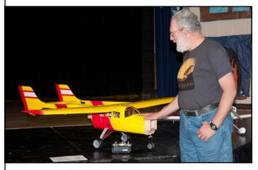
**Wade Wiley – Nitro Planes** – Spymasters set up as a camera plane motor equv. 120 or 1500 watts, setup with flight 3 axis flight stabilization camera to be 90-120 Wide angle
