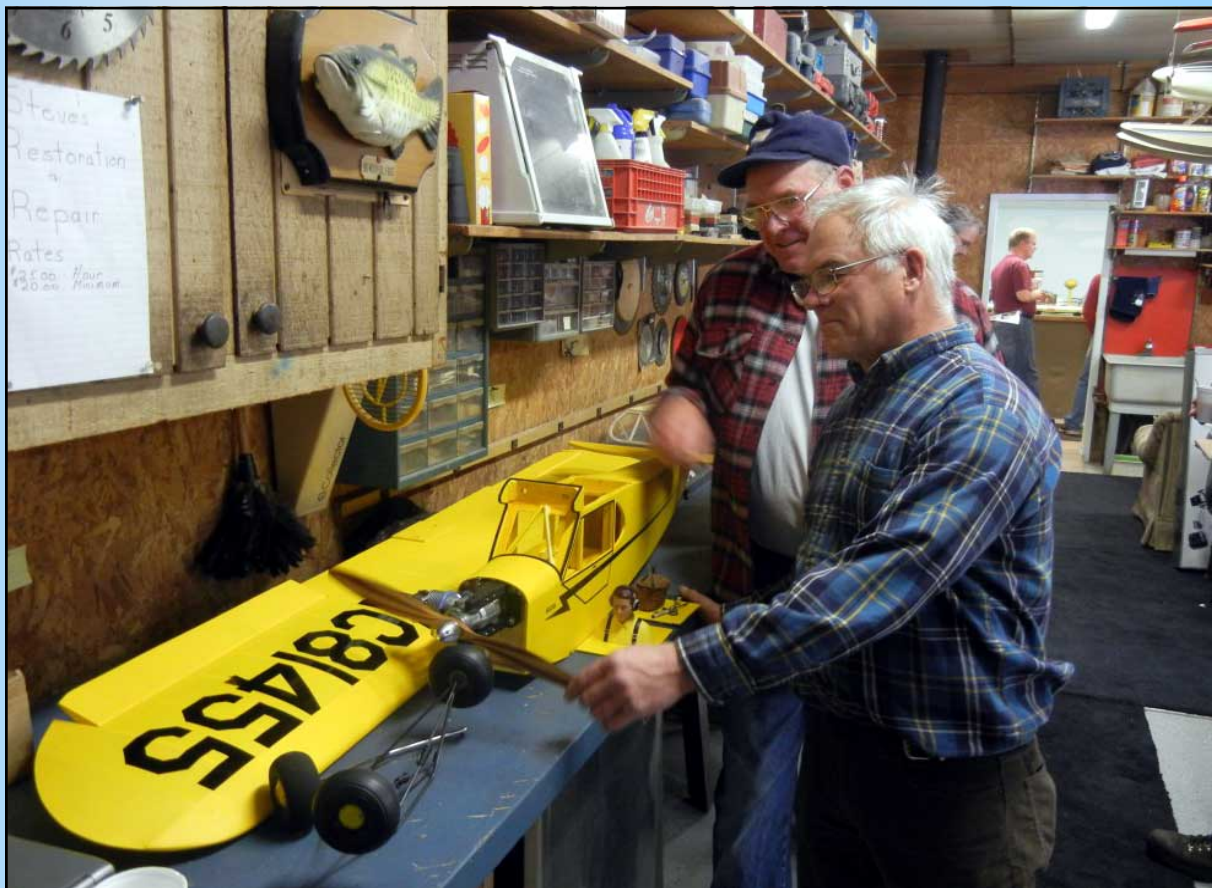
Steve Fredericks talks to Bill Dezur about his Piper J3 Cub - ¼ scale, with 81" wing span, covered with Yellow Cover Rite and will be powered by a Saito 80.
