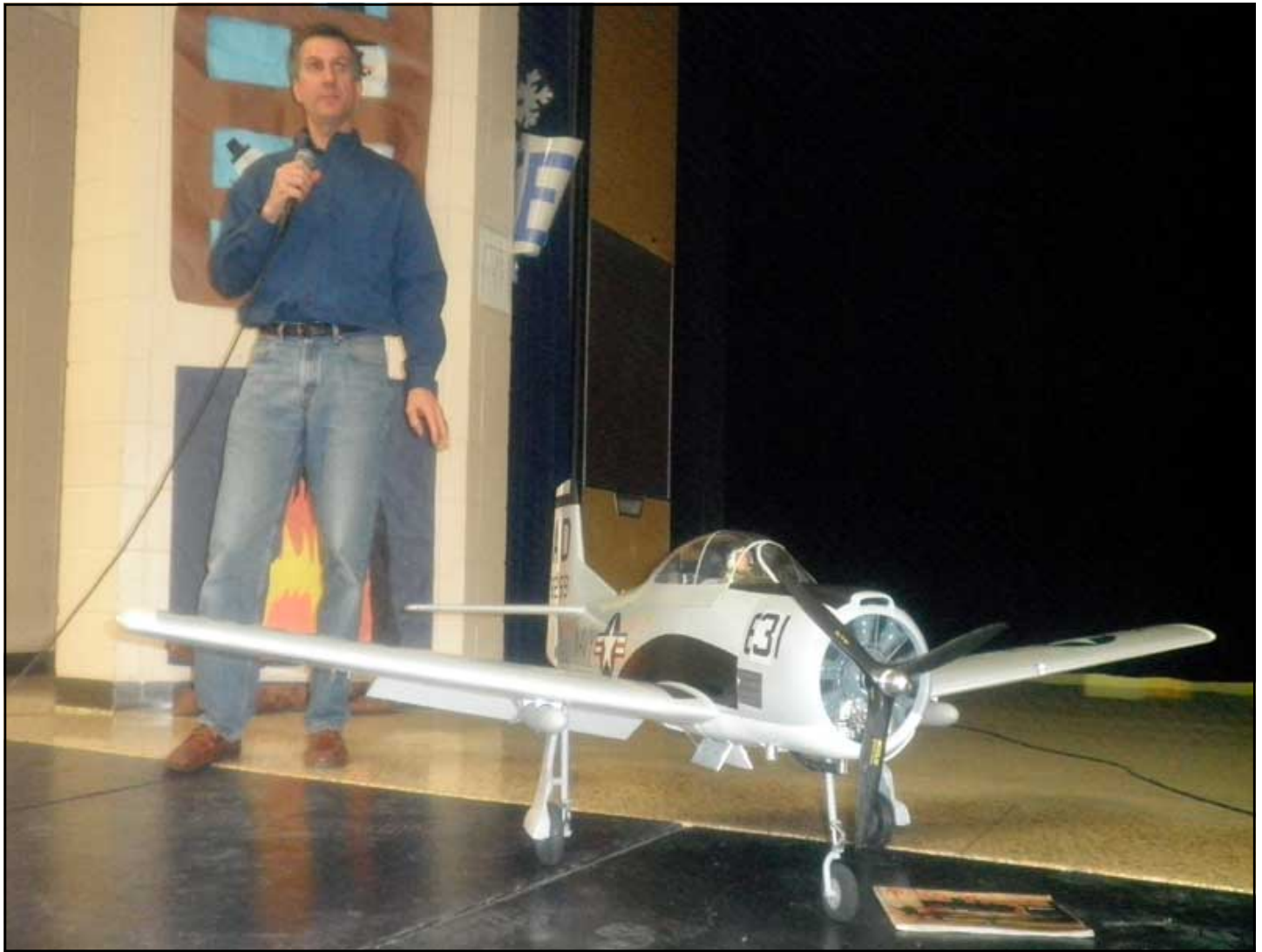
Gary Weaks brought in his beautiful North American T-28 B, plan-built from Dave Platt plans. WS is 81", Weight 17.5 lbs, engine is an Evolution 40 cc gas. The plan has retractable gear, working flaps and releasable bombs. It is finished with Ultracoat.
