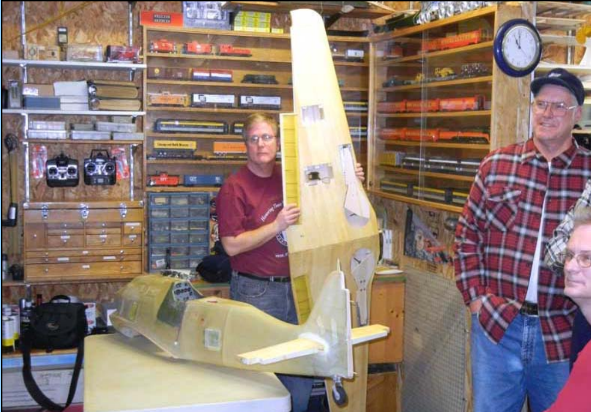
Joe Finkelstine's ~ Focke-Wulf 190 A8, 1/5 scale, powered by a 450 - 3 cylinder, fiberglass skin, will be painted with Glass Coat Epoxy.
