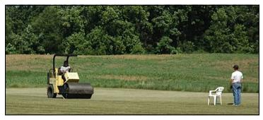
A little piece of trivia about the roller: The roller weighed 6,800 lbs but when in vibration mode it provided 15 tons of compaction to the field.
