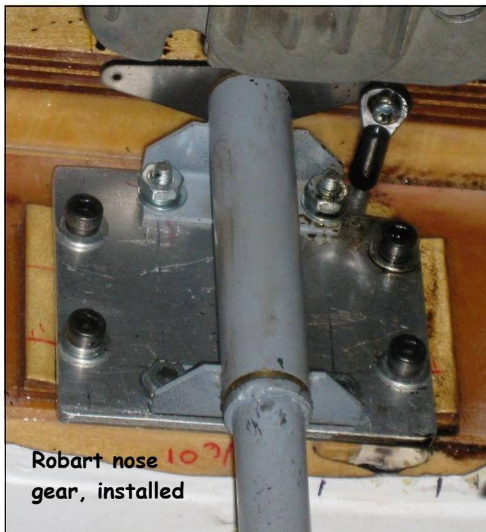
All nose gear maintenance can be performed by just unbolting the plate, and repairs can be easily handled by ordering parts from Robart.
