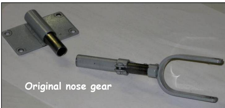
Upon internet research, I found that Robart makes a large scale steerable nosegear with comparable dimensions, product number 159F. To mount the Robart gear, all that was needed was an adapter plate. This was constructed from 1/8" aluminum.
