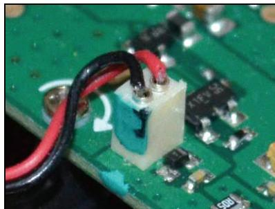
motor connectors closest to each boom. Observe polarity... the negative (black) motor wire goes in the side of the board connector that has the green mark on it.
