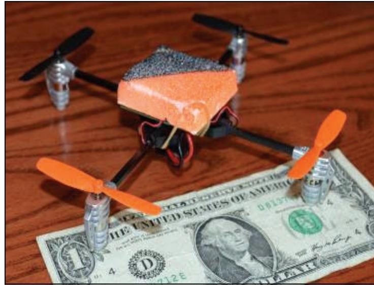
I made my canopy from a small block of styrofoam, to protect the motor wires (I didn't use the adapters). You can also make one from the bottom of a water bottle. Keep it VERY light though.... Every gram counts.
