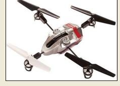
and inertia. Oh, and maxed out control throws. Mine are set to 150%. And never exceed 90% throttle for more than a second or two or it will become unstable.
