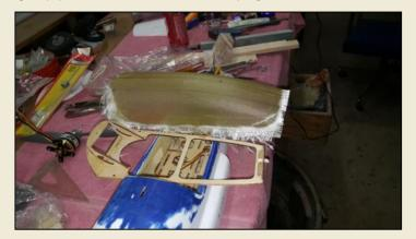
In last months article you will recall that we applied the yellow tape to mark where we will trim the part. Although not visible in this picture the yellow tape left a clear ridge on the inside of the part. This is where the part gets trimmed. The glass is pretty thin and is easily trimmed with a pair of scissors. Once trimmed I sand the inside surface of the
