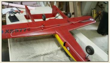
Make a loop of string or cord (depending on the weight of your model). Use the lightest cord that can safely support your models weight. The length will be determined by the size of your model.
