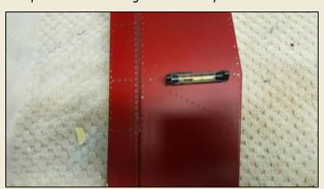
If you don't have a nice spot to put the plastic level I have also used the horizontal stabilizer to level the model. Just make sure that you remove it before you take your cg location. Use the level for consistency between adjustments.
