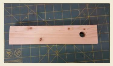
Drill a hole the size of your dowel near one end of the larger piece of 1X2. Make sure the hole is on the long center line. The dowel should be a snug fit but be able to rotate in the hole.
