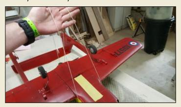
Now take the loop and slip it over the nose and the rear portion of the fuselage. In this example it is around the nose and the prop shaft of the pusher motor. The exact location doesn't matter as long as the front portion is
