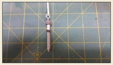
Using the 12" piece of string make a loop through the end of the plumb bob. I made the loop the same way as I did with the heavy cord.
