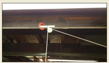
Attach the small block to something solid above your bench, hang the pulley from the screw you put in the block and run the heavy cord through the pulley. Tie off the loose end of the heavy cord to something solid.
