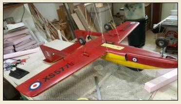
Now using the heavy cord lift the model off of your bench a couple of inches and secure the cord to keep the model in the air. Now adjust the length of the plumb bob string so that the bob is just above the surface of the model. Now we want to level the model. Loosen the 1/4-20 friction bolt and rotate the dowel to bring the model to a level flight attitude. To be consistent with this I use a small plastic line level resting on the bottom of the fuselage as in the picture below.
