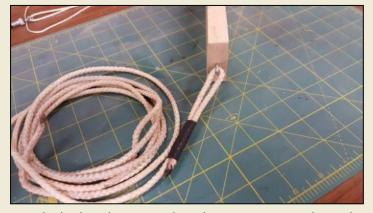
Attach the long heavy cord to the screw eye on the end opposite from the dowel hole. I made a loop and bound the joint with light string. I applied CA clue to the joint then put a piece of shrink tube over the joint.
