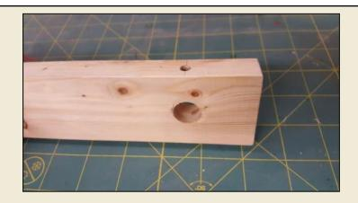
Drill and tap a hole for the 1/4-20 bolt in line with the dowel hole. Thread the bolt into the hole. This bolt will lock the dowel from turning when it is installed.
