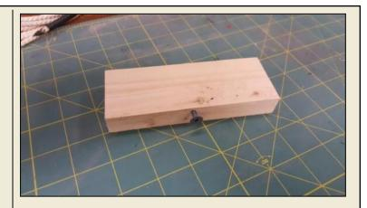
Here is the small block with the wood screw installed. The pulley will be hung from the screw and the whole thing will be clamped to a joist or beam above your work bench.
