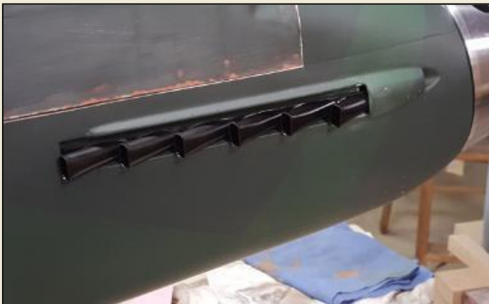
Stacks mounted on fuselage
