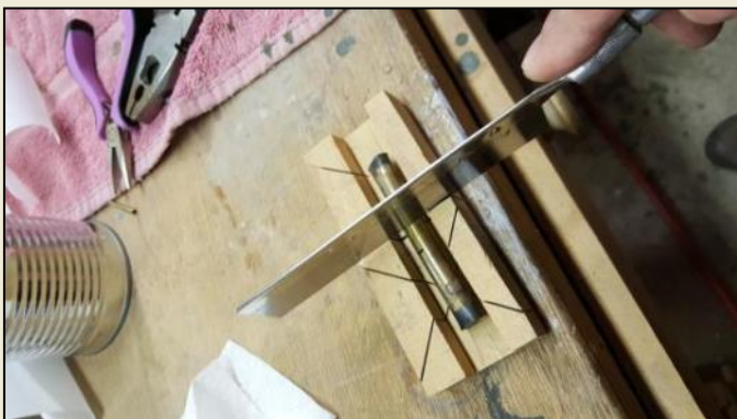
Cut tube to length with razor saw
