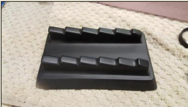
Vacuum formed exhaust stacks
