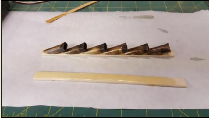
Stacks epoxied to the wood mounting strip
