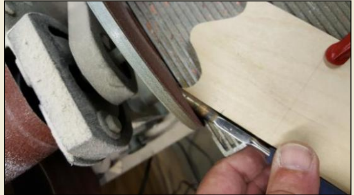
Shaping the angle using a disk sander and scrap wood guide
