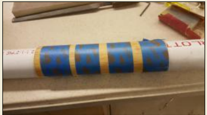
Wet balsa taped to PVC pipe
