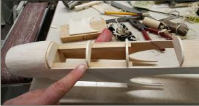
Extra bulkhead added for support
