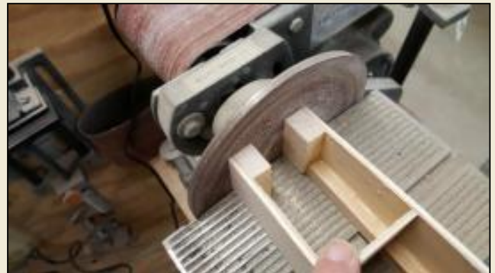
Sanding the 3 degree angle
