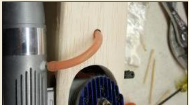
Pressure line exit from bottom block
