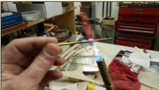
Annealing the brass fuel tube
