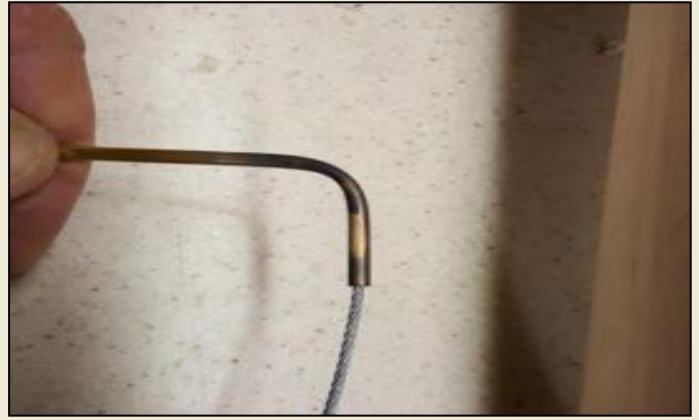
Steel cable prevents total collapse of tube
