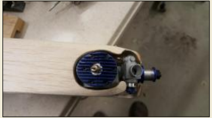
Cylinder and carburetor clearance
