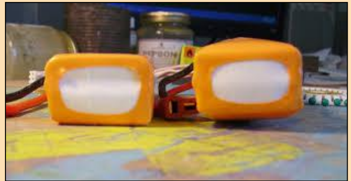
Good pack (left) vs. puffed pack (right)
