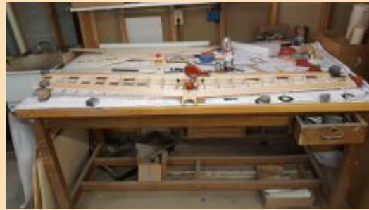
Trial assembly of the two wing panels.
