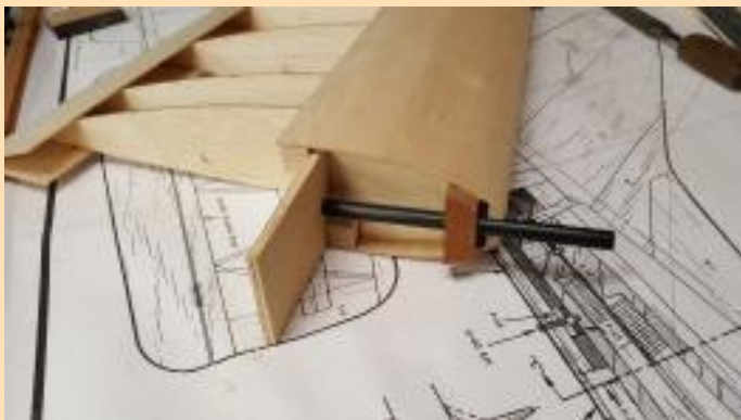
Leading edge pin, support block, half ribs and dihedral brace.
