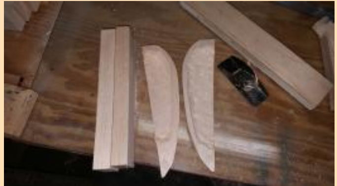
Hollowing out the wing tip blocks.
