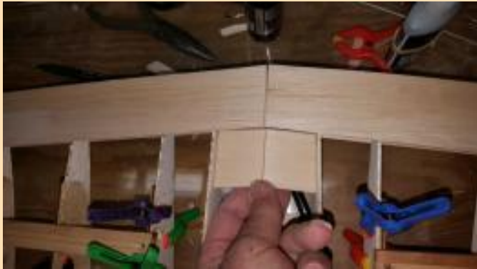
Wing bolt reinforcement being installed.
