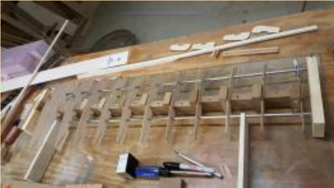
Ribs and spacers on jig.
