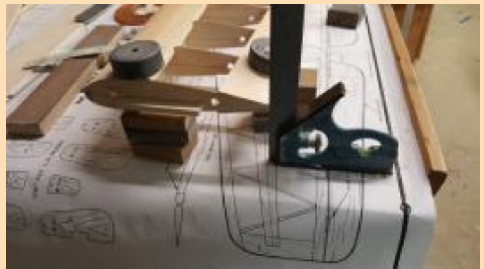
Left tip rib cord line height check.
