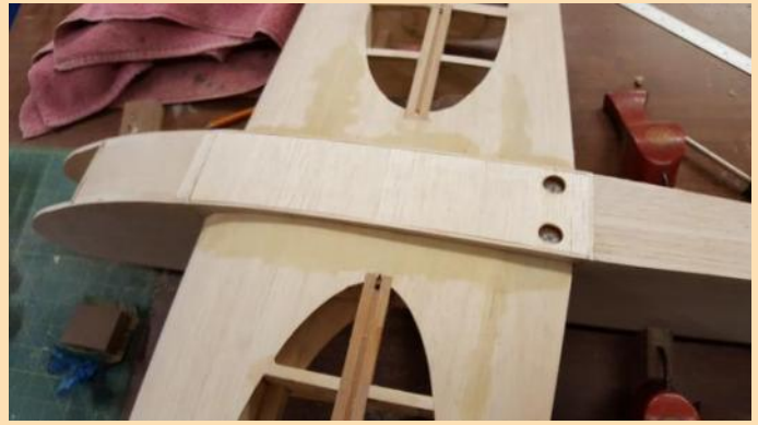
Belly pan installed
