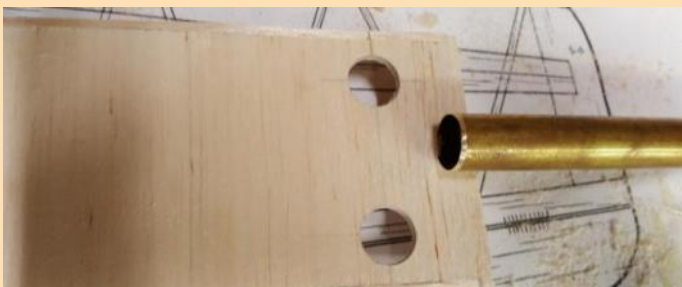
Locate and cut holes for wing mounting bolts
