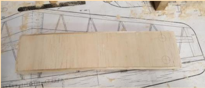
Filling with 3/32" sheeting
