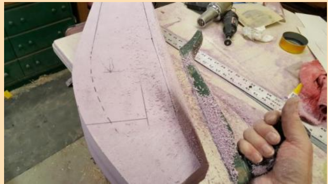
Tangent lines and Sureform file work
