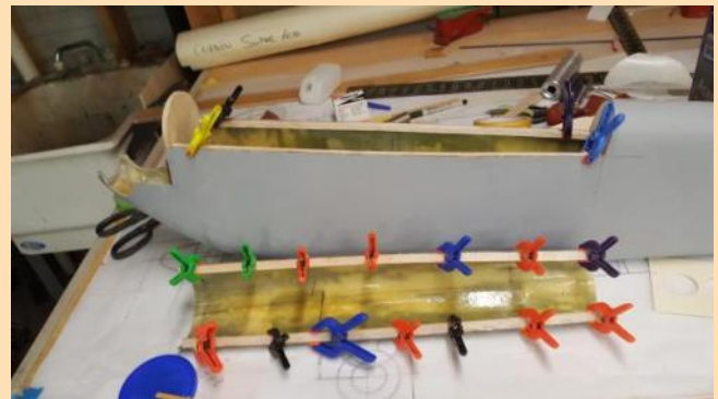
Adding stiffeners and bulkheads
