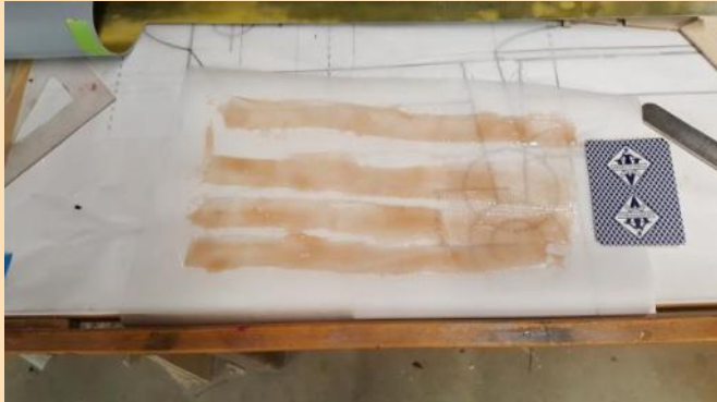
Bottom seam repair glass strips
