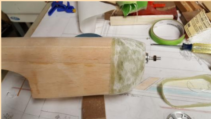
Fiberglass after rough sanding
