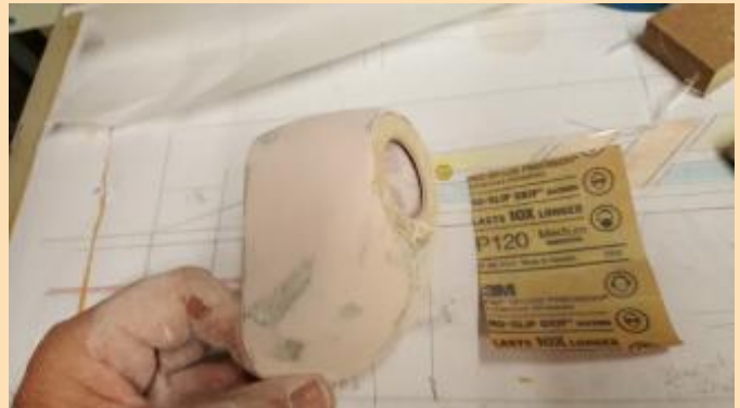
Spot putty sanded and ready for primer
