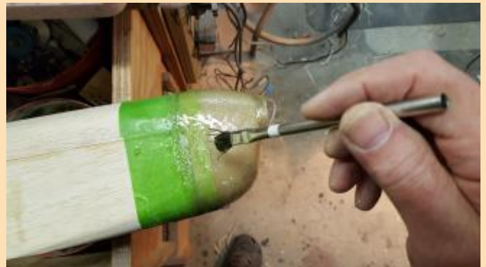
Two layers of fiberglass being applied
