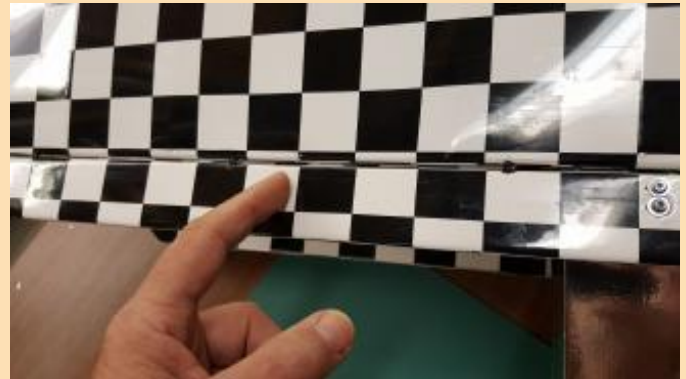
Pattern match at trailing edge to flap
