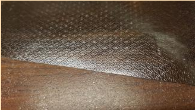
Air passages on back of the vinyl.
