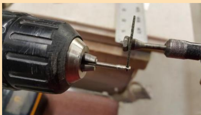
Grooving the gear down indicator wire pin.
