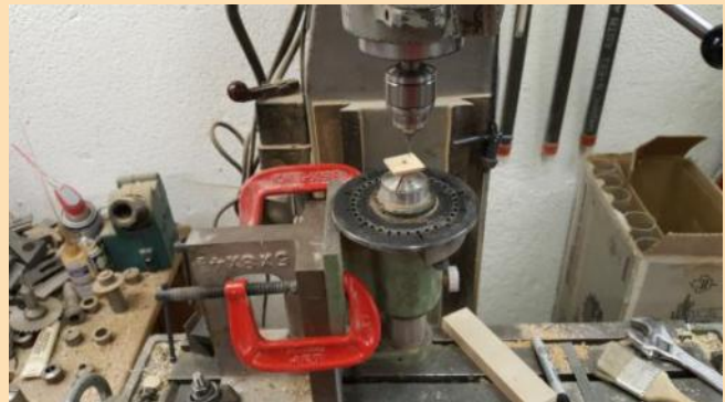
Drilling 12 equally spaced holes.
