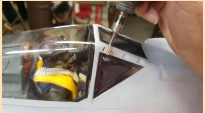
Cutting recesses for windscreen armor clamp bolts.
