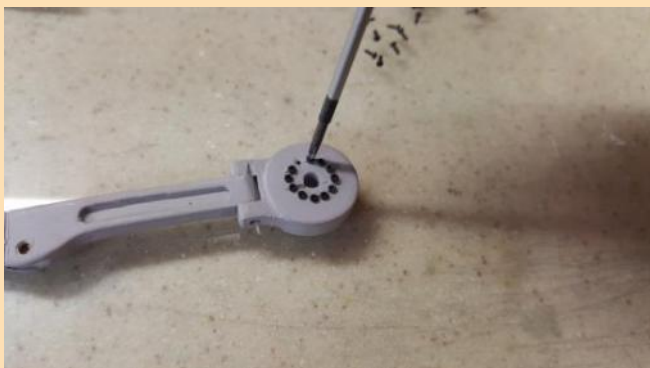
Installing the screws in the retract motor.
