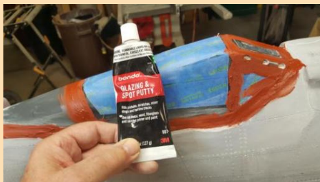
First layer of Bondo #907 before sanding.
