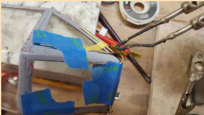
Old canopy used as a soldering fixture.
