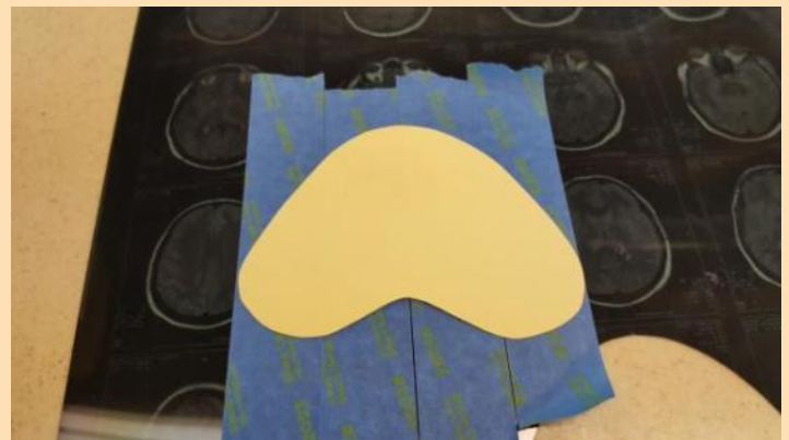
Marking the cut line for the windscreen.
