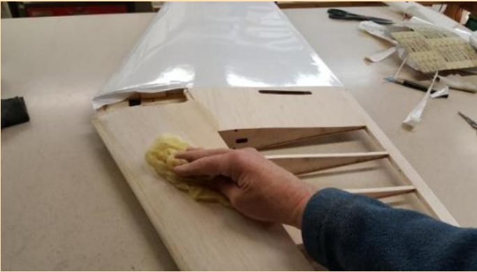
Using a tack cloth to clean the surfaces.
