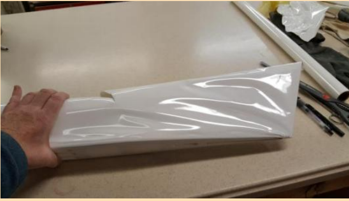
Side covering ready to be shrunk.
