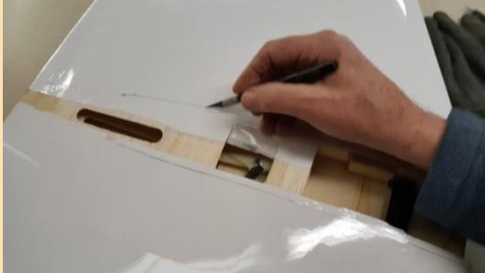
Cutting the covering at the marked line.
