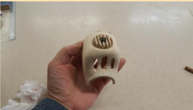
Cowl ready for covering.
