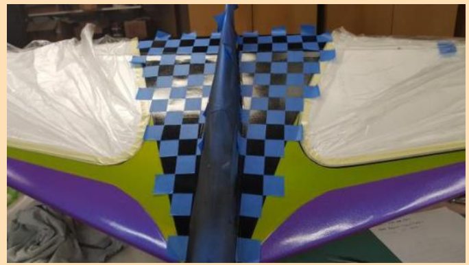
Checkerboard masking is complete.
