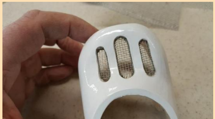
Covered cowl with screen inserts installed.
