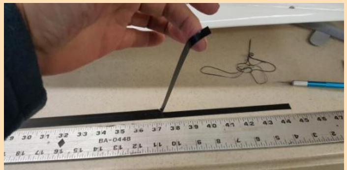
Cutting electricians tape into narrow strips.
