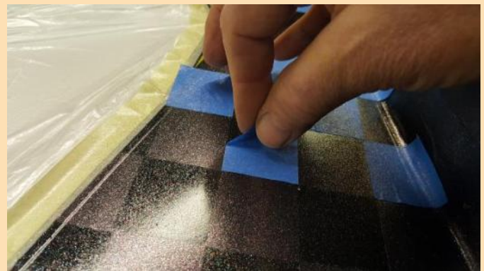
Removing the checkerboard masking.
