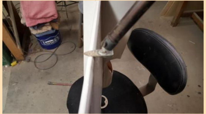
Fusing the covering film into the hinge recesses.
