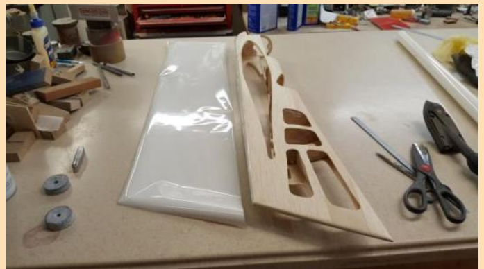
Fuselage side covering piece is cut about an inch oversized.
