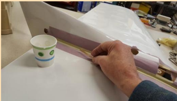
Applying epoxy into the fuselage to wing joint.
