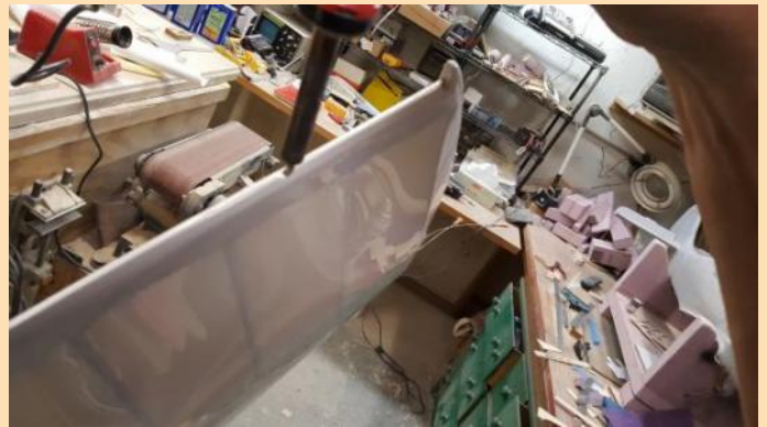
Melting the film blocking the hinge hole.
