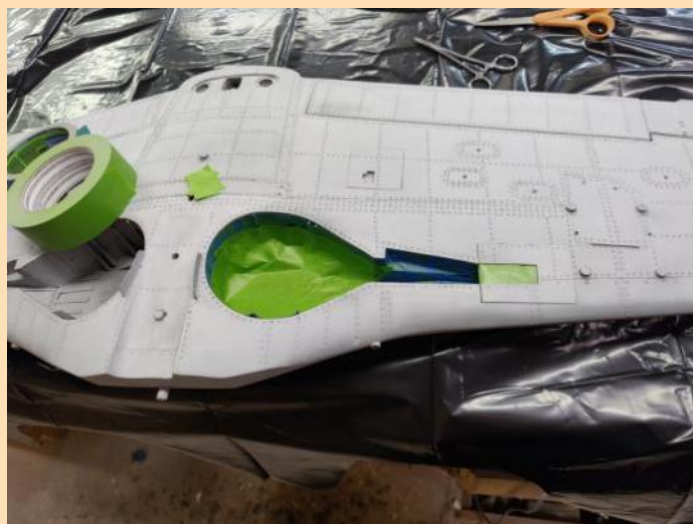
Masking the inside of the wheel wells.
