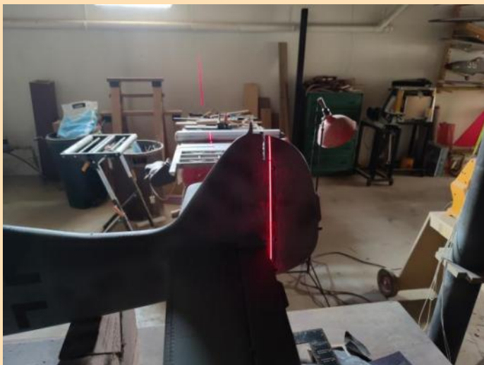
Laser aligned with the rudder hinge line.
