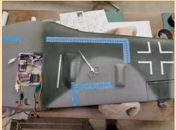
Dashed line masking in place.
