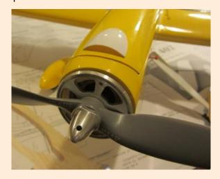
To allow air into the motor bay I had to cut an opening on the motor hatch which roughly followed the profile of the spoon.
