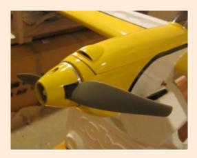
The motor still runs a little warmer than I would like so I might add a small baffle under the scoop to direct more air onto the motor but for now the situation is much improved.
