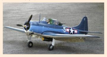
The model is large with a wingspan of 81", a wing area of 1300 sq in and a finished weight of about 15.4 lb. At that weight the wing loading approaches 28 oz per sq foot; it is on the heavy side. Most of our aerobatic or sport models have wings loadings in the 23 oz range. It will need to be flown with care.
