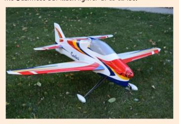
In this case the recommendation would remain the same, an 85 pack swinging a 18x12 prop should fly the model well.
