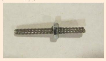
The next step is to glue the adapter in place. I have had good luck using 30 minute epoxy although some prefer to use JB weld.
