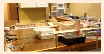
Once the components are aligned, I tack glue them in place using a drop of CA here and there and then recheck everything to make sure that nothing shifted. Once satisfied I epoxy the components in place. You can save a little weight by adding micro balloons to the epoxy. Doing this has the added benefit of making the epoxy a little easier to sand. I always allow the epoxy to set overnight; I just want to be sure that it is fully hardened before I handle the model once again.
