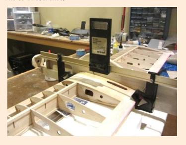
On a profile model it is difficult to change the incidence of the wing without enlarging the opening significantly, so I opted to set the stab relative to the wing. I used the incidence meter determine a datum for the wing and then set the stab relative to it. As you can see from the image below, I had to shim the stab to achieve the proper angle.
