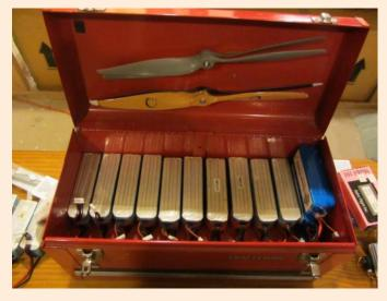
Shown in the picture are enough packs for six flights on the Vanquish (10S) or twelve flights (5S) on one of the smaller models.
