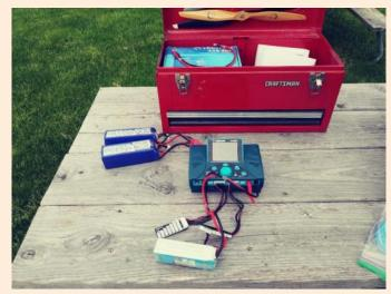
The smaller C/L models use a 45 2600 mah pack while the larger ones use a 65 2200 mah pack. The set up allows me to charge the 45 packs five times or three times for the 65 packs. Enough for a day of flying.
