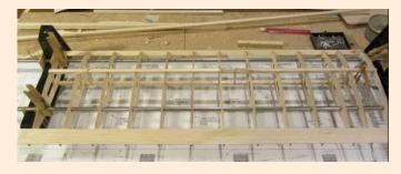
I use rubber bands to hold the spars and leadingedge pieces in place as well. Once satisfied that everything is lined up correctly and level, I glue it up using thin CA. A panel can be framed in about 1 hour. If necessary, I use old playing cards to shim the brackets to make sure that the wing panel is straight and level.
