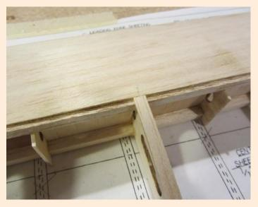
The reason for this is simple, the exposed portion of the spar provides a surface for the 1/16" ribs caps to rest upon. By doing this the rib caps will always be perpendicular to the rib.
